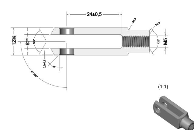
No sharp ends, no burrs, no significant surface defects. General Tolerances DIN ISO 2768-medium
