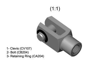
No sharp ends, no burrs, no significant surface defects. General Tolerances DIN ISO 2768-medium
